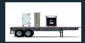
**Exact equipment specification** of each vehicle/container/substation including one or more of the following key components: HV/MV switchgear, power transformer, protection and control panels, auxiliary AC&DC services, HV/MV cable and reels and system control equipment.
